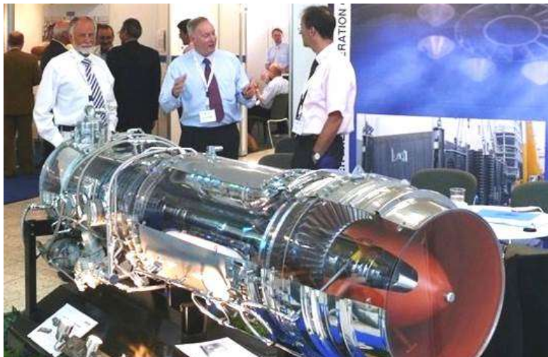
Cut-away Gas Turbine ROLLS ROYCE KB5 in the Zellcheming Fair in Wiesbaden, Germany
